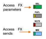
Access FX parameters from the strips Press an FX send master strip SEL key, or press an FX short return (IP FX) strip SEL key to open up the FX screen. You can adjust the parameters (Front Panel view), configure the routing (Back Panel view) and work with libraries.
